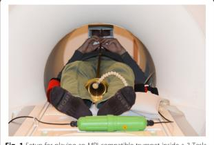
Fig. 1 Setup for playing an MRI-compatible trumpet inside a 3 Tesla MRI system
