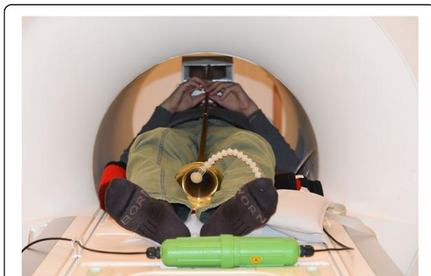
**Fig. 1** Setup for playing an MRI-compatible trumpet inside a 3 Tesla MRI system
